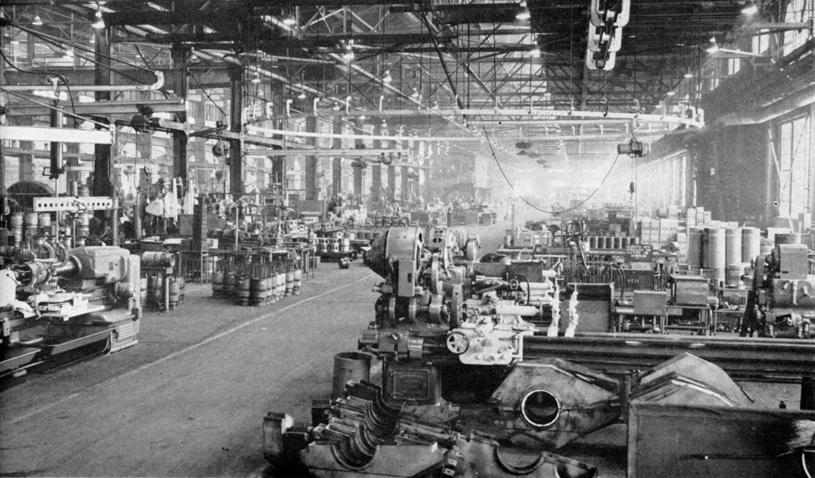
Liner reclamation is handled in the area at the center. Behind and to the right is the conveyor system for heads. Post cranes and tramrails facilitate materials handling at various steps in the processes.
